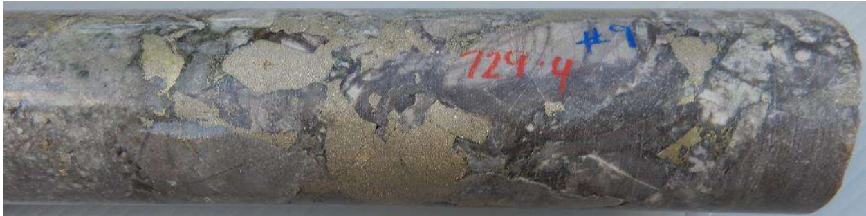
Fig 19 HQ Core photo hole 21CAEDD009, 729.4m Highly sulphidic clast supported breccia. Polymict clasts dominated by hornfels. Abundant pyrite, moderate chalcopyrite infill. 729-730m assays 1m @ 0.27% Cu, 0.30 g/t Au, 8.4 g/t Ag, 8.5 % S.
