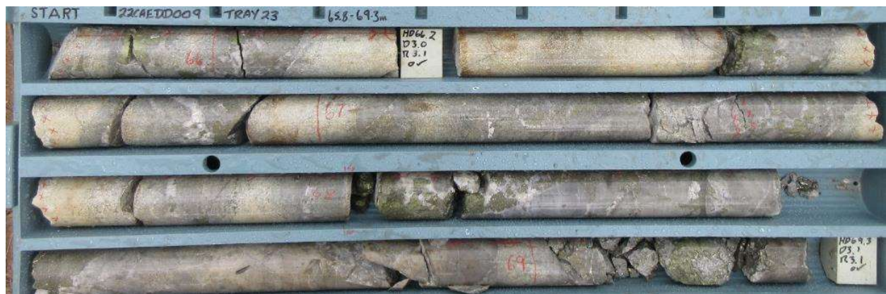
Fig 10 HQ Core photo hole 21CAEDD009, 65.8m to 69.3 Chalcopyrite -pyrite infill in hydrothermal diorite dominated breccia. Primary zone 65m-70m assays 5m @ 1.70% Cu, 0.42 g/t Au, 30.3 g/t Ag, 9.48 % S.
