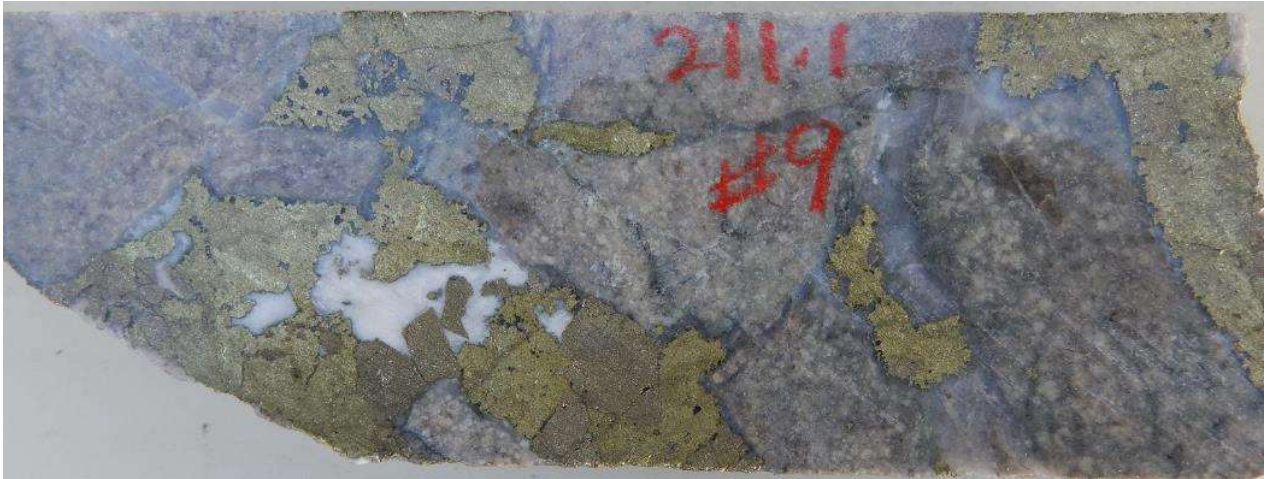
Fig 15 HQ Core photo hole 21CAEDD009, 211.1m Chalcopyrite pyrite calcite quartz infill in hydrothermal diorite dominated breccia. Primary zone 211m-212m assays 1m @ 4.69% Cu, 0.78 g/t Au, 58.5 g/t Ag, 7.90 % S.
