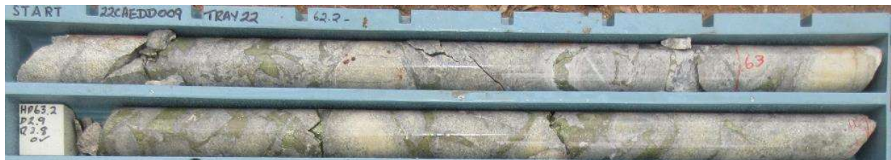
Fig 8 HQ Core photo hole 21CAEDD009, 62.3m to 64m. Chalcopyrite rich infill in hydrothermal diorite dominated breccia. Primary zone 62m-64m assays 2m @ 2.88% Cu, 0.53 g/t Au, 41 g/t Ag, 8.91 % S.
