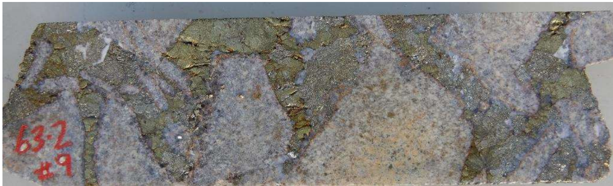
Fig 9 HQ Core photo hole 21CAEDD009, 63.2m Chalcopyrite -pyrite infill in hydrothermal diorite dominated breccia. Primary zone 63m-64m assays 1m @ 3.89% Cu, 0.78 g/t Au, 58.8 g/t Ag, 11.83 % S.
