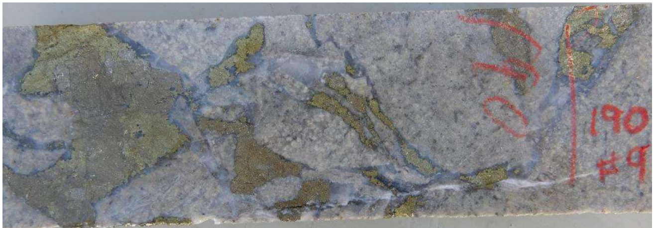
Fig 12 HQ Core photo hole 21CAEDD009, 190.0m Chalcopyrite -pyrite infill in hydrothermal diorite dominated breccia. Primary zone 189m-190m assays 1m @ 2.09% Cu, 0.20 g/t Au, 31.5 g/t Ag, 7.25 % S .
