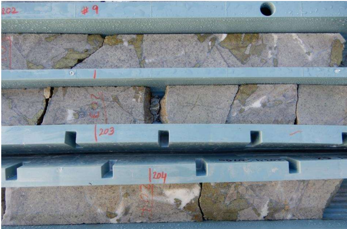
Fig 13 HQ Core photo hole 21CAEDD009, 202m-205m Chalcopyrite -pyrite infill in hydrothermal diorite dominated breccia. Primary zone 202m-205m assays 3m @ 2.53% Cu, 0.58 g/t Au, 48.7 g/t Ag, 5.27 % S.
