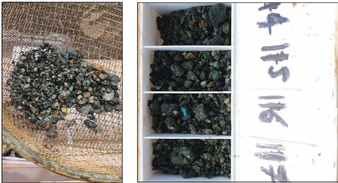
Fig.1 Section of visible copper mineralisation intersected in RC drilling (WGR0350, 114-118m)
