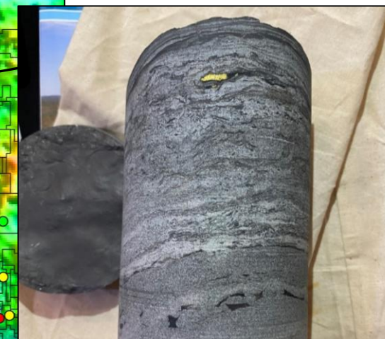
Chalcoprite contained in a calcareous shale unit within NDI Carrara 4
