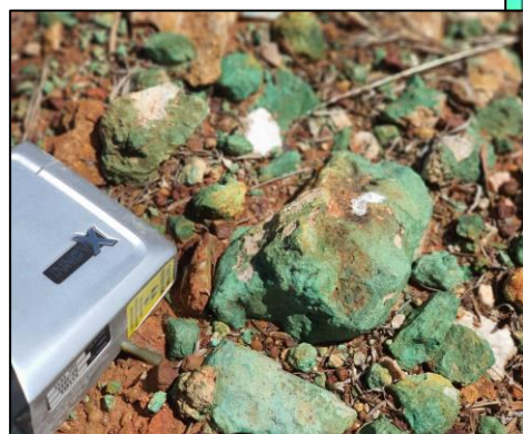
Crosswinds Copper Prospect – Malachite (copper carbonate) mineralisation exposed in table drain 2
