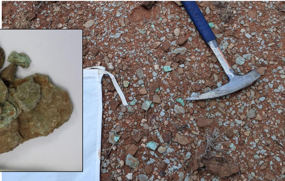
SA0000011 selected sample of surface scree Sandover 5.5% Cu (Area 2)
