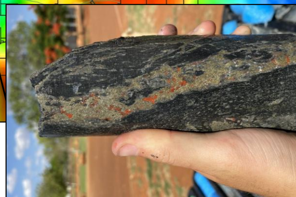
Drill hole NDIBK04 pyrite- chalcoprite vein 3
