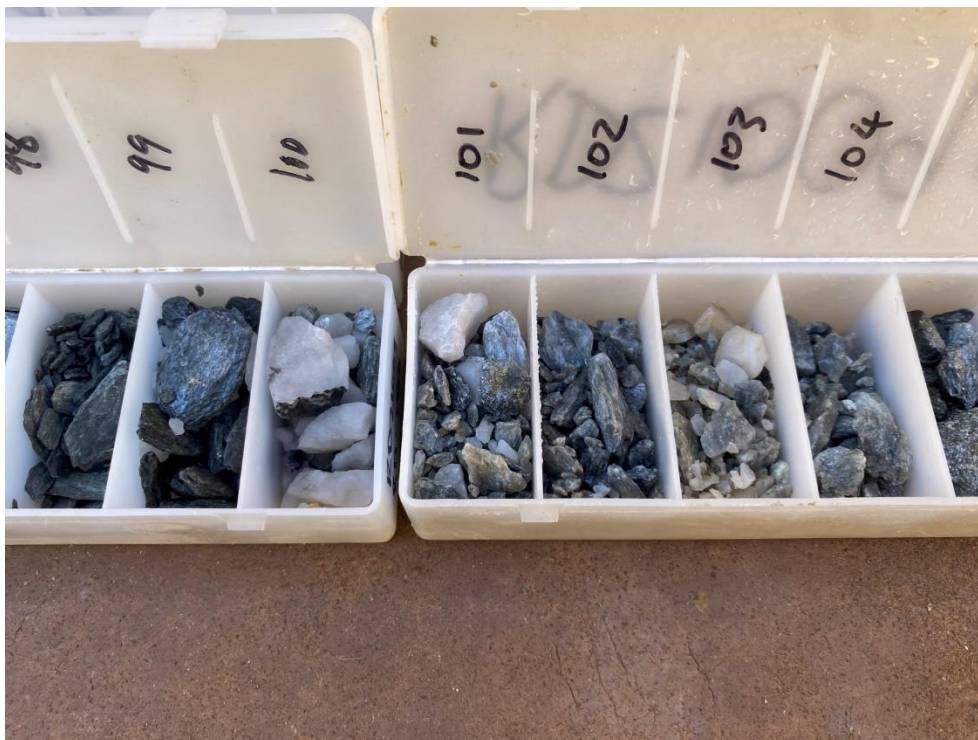
Figure 2. Photograph of RC drill chips from RD21009 (97 – 104 metres) showing visible sulphide and quartz veining present
