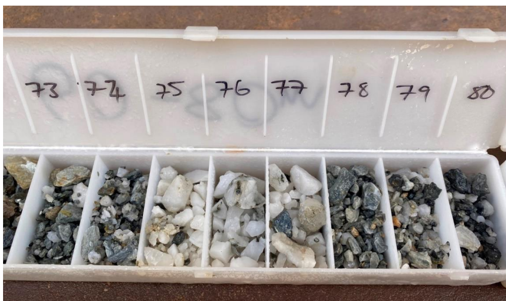
Figure 3. Photograph of RC drill chips from RD21008 (72 – 80 metres) showing quartz veining and sericite \pm chlorite alteration
