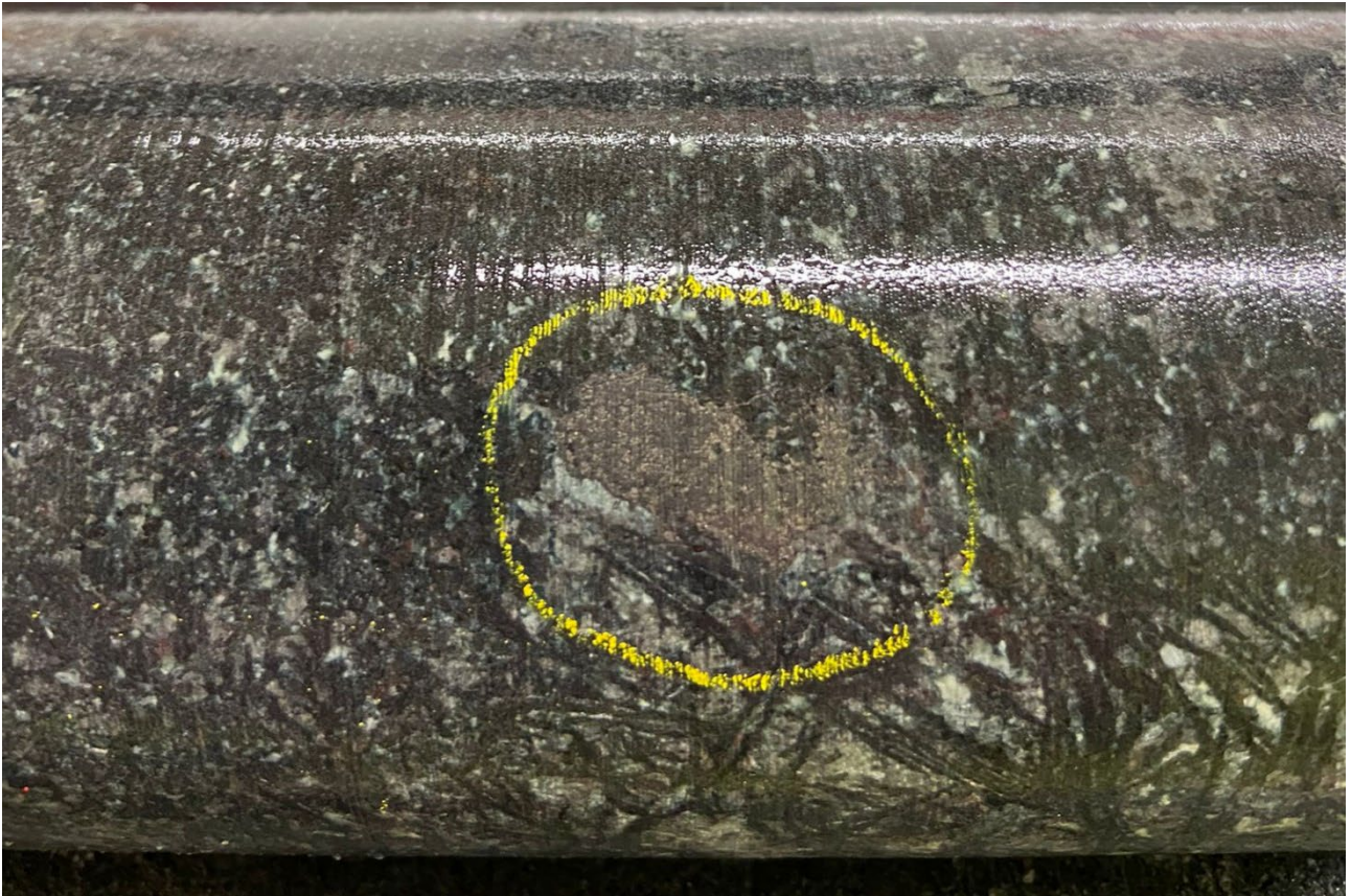
Figure 4: DDED22-085, Blebby heazlewoodite-millerite within pyroxenite at 150.24m
