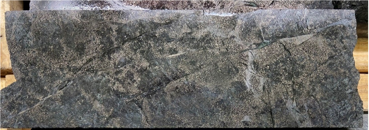
Figure 6: DDED22-085, disseminated heazlewoodite-millerite within pyroxenite at 270.4m
