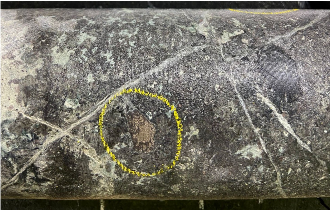
Figure 5: DDED22-085, Blebby heazlewoodite-millerite within pyroxenite at 151.34m
