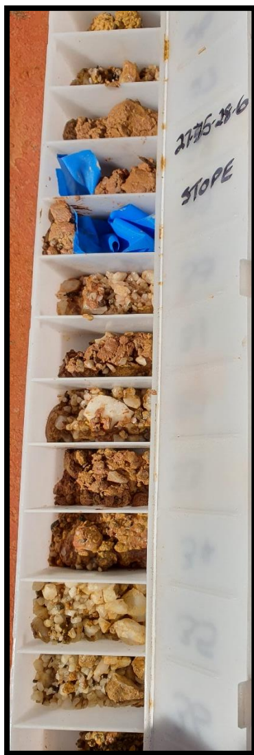
Photo 1: Chip Tray of RRC070 26-33m showing stope (in blue) and strong quartz veining below
