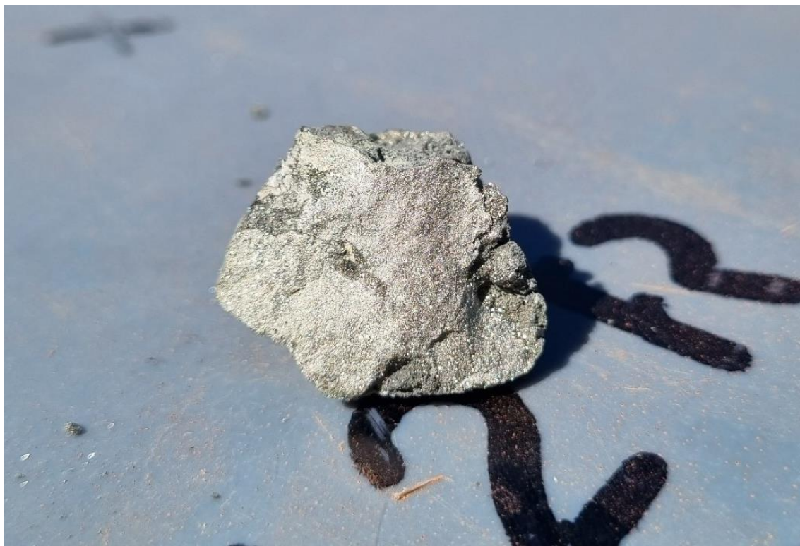
Figure 3. Massive sulphide sample from 49-50m in GJAC562, (3m @ 3.00g/t Au and 17.2g/t Ag)
