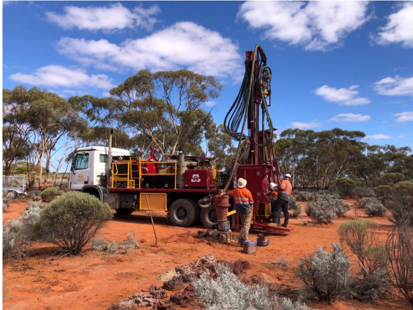
Figure 4. Aircore drill rig at Blackfriars target.
