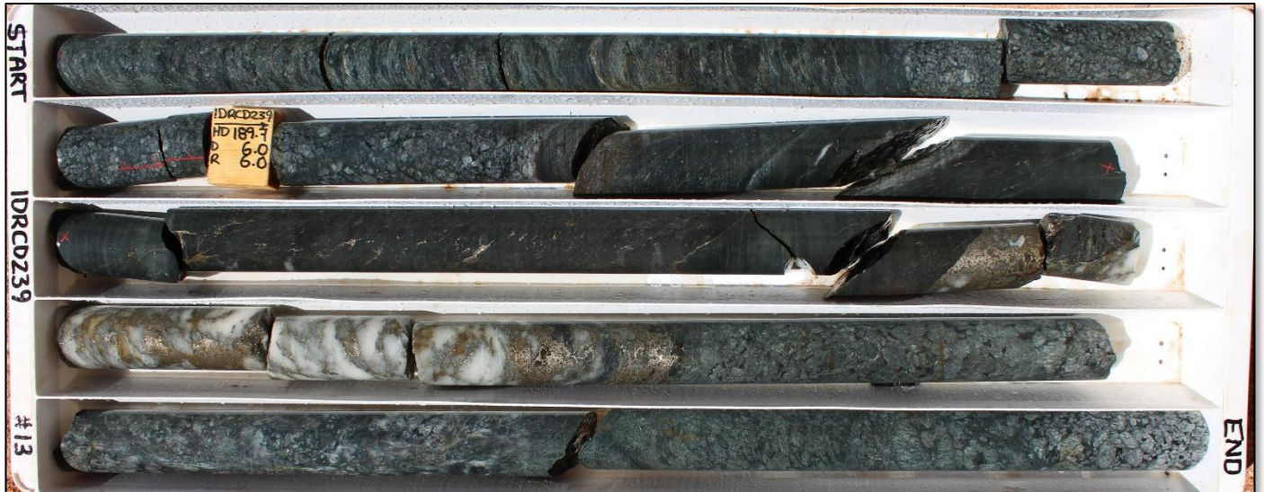
Figure 10; IDRCD239 diamond core interval showing strongly mineralised quartz veining with massive and semi massive sulphides in a sheared mafic and Anorthosite host interval from 190m to 192.3m#
