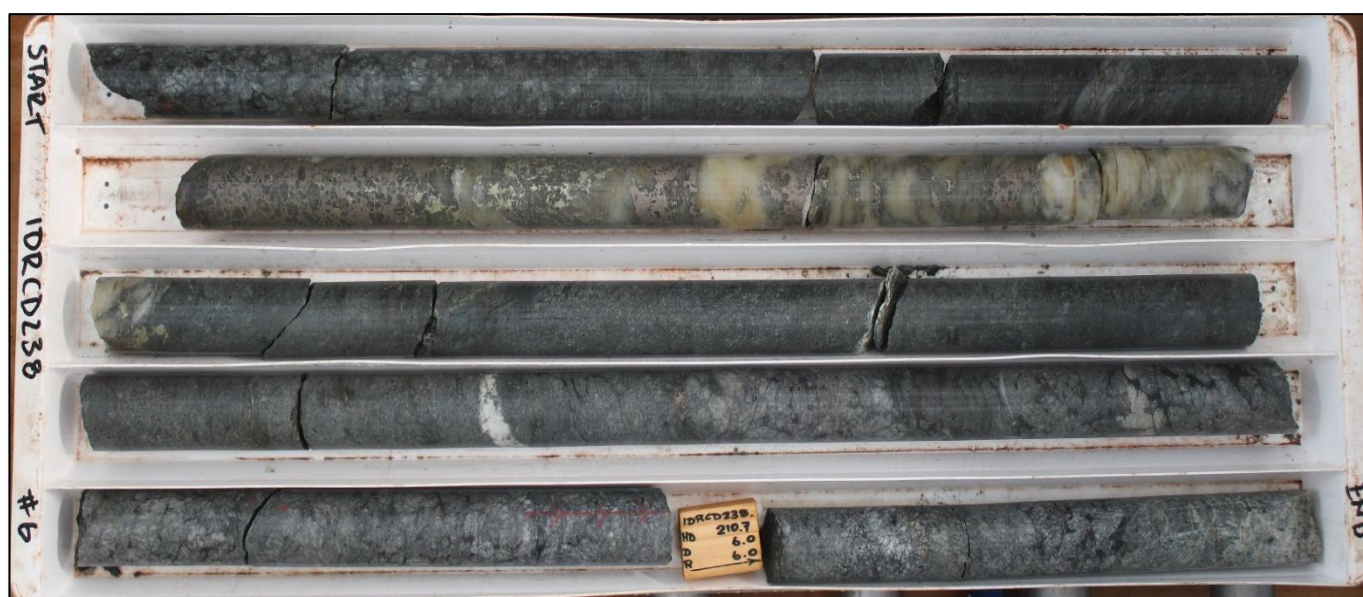
Figure 9; IDRCD238; Uncut diamond showing 1.2m of semi-massive sulphide (Pyrrhotite and Chalcopyrite) in quartz veining within and Anorthosite country rock (206.9m to 208.3m) #
