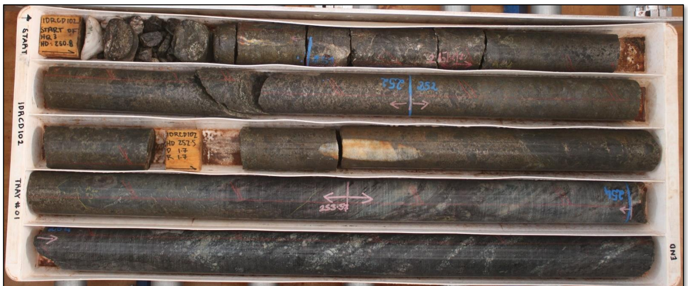
Figure 11; IDRCD102 HQ drill core intersected massive to semi massive sulphides predominantly pyrrhotite, pyrite with minor Chalcopyrite from 250.8 to 253.7m #
