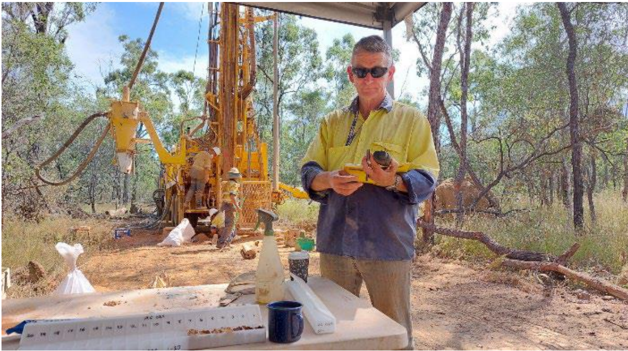
Image 3: Chip tray samples being collected from RC drilling program at Gunnawarra
