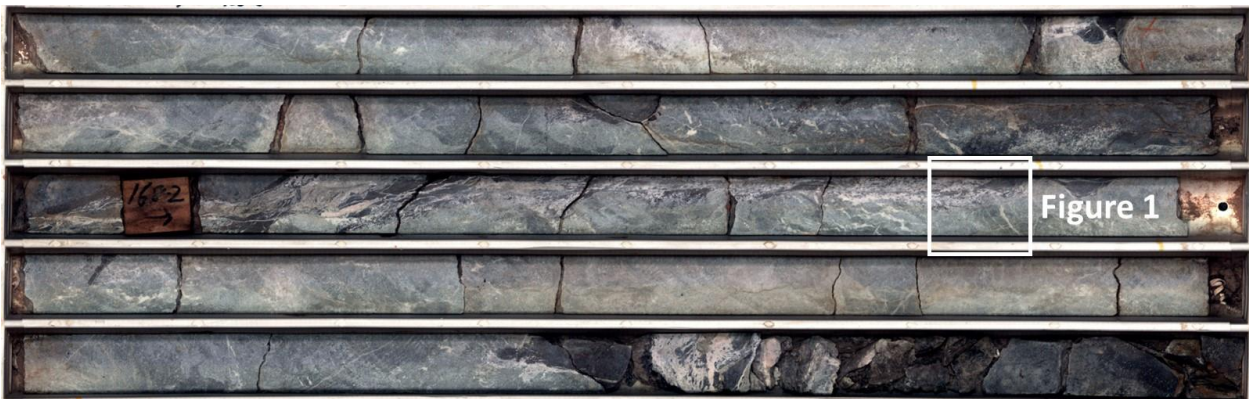
Figure 4: MWDD002 166.2m to 170.9m showing intense silica and carbonate alteration. The location of Figure 1 from the first page of this announcement is also shown.
