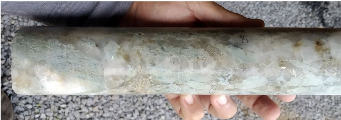
Figure 4: Green spodumene associated to quartz and some feldspar and mica at 62.5m depth in SADD011
