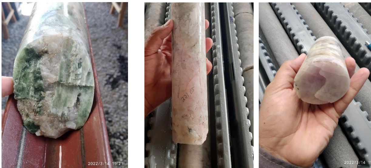
Figure 1: Green and light pink-purple spodumene crystals in drill core from SADD006 (assay results pending)
