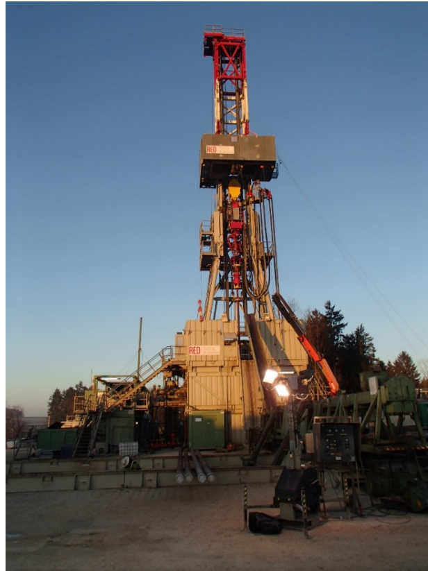
Running casing using the RED E-200 rig at the Anshof-3 drill site
