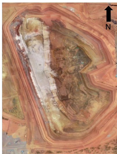
Photo: Mt Weld open cut mine as at 1 April 2022 showing benches of waste removed from Campaign 4-1 to the west (left of image)
