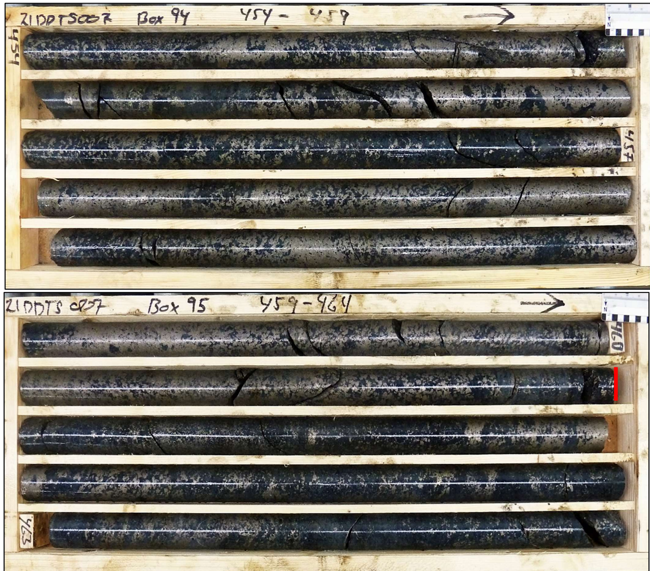
Figure 2: Magmatic Ni-Cu sulphides in 21DDTS007 displaying massive to semi-massive and matrix to coarse blebby sulphide mineralisation within the core of the host gabbroic intrusion. Assays returned 7m @ 1.57% Ni, 0.52% Cu & 0.13% Co (454-461m) and typical mineralisation below the higher-grade zone (461-464m).
