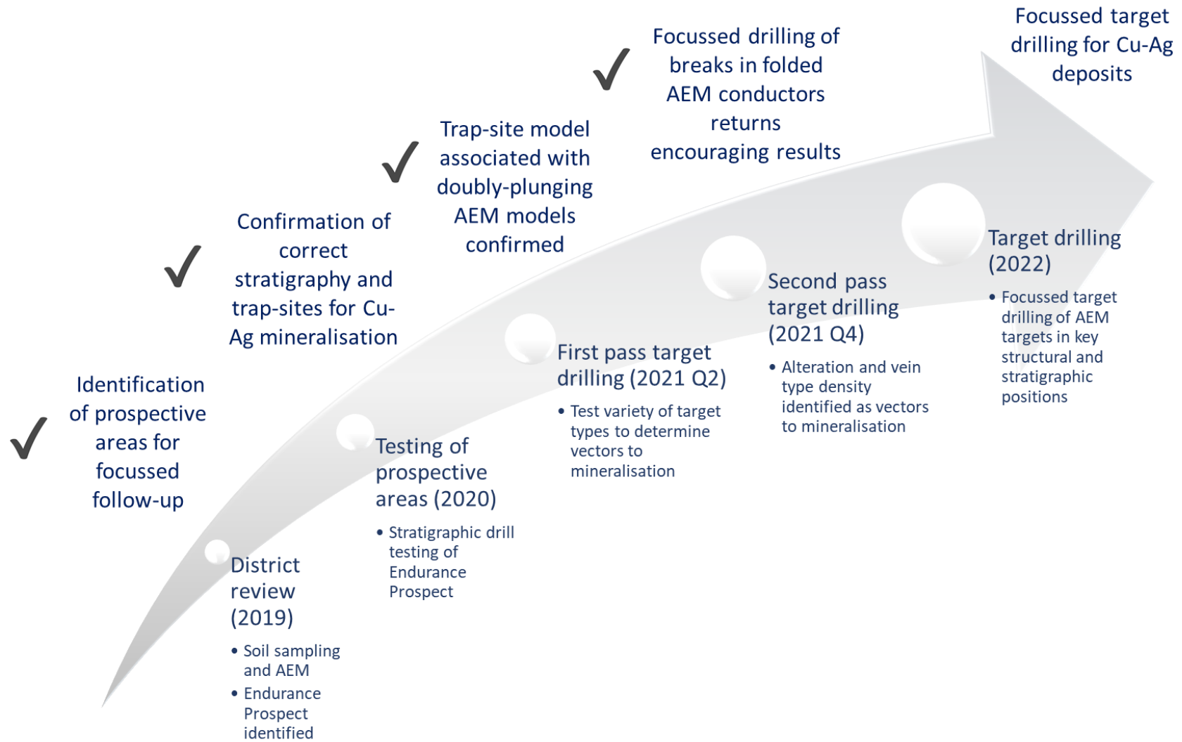
Figure 3. Summary of exploration phases over the Endurance Prospect leading up to the proposed 2022 drill programme.
