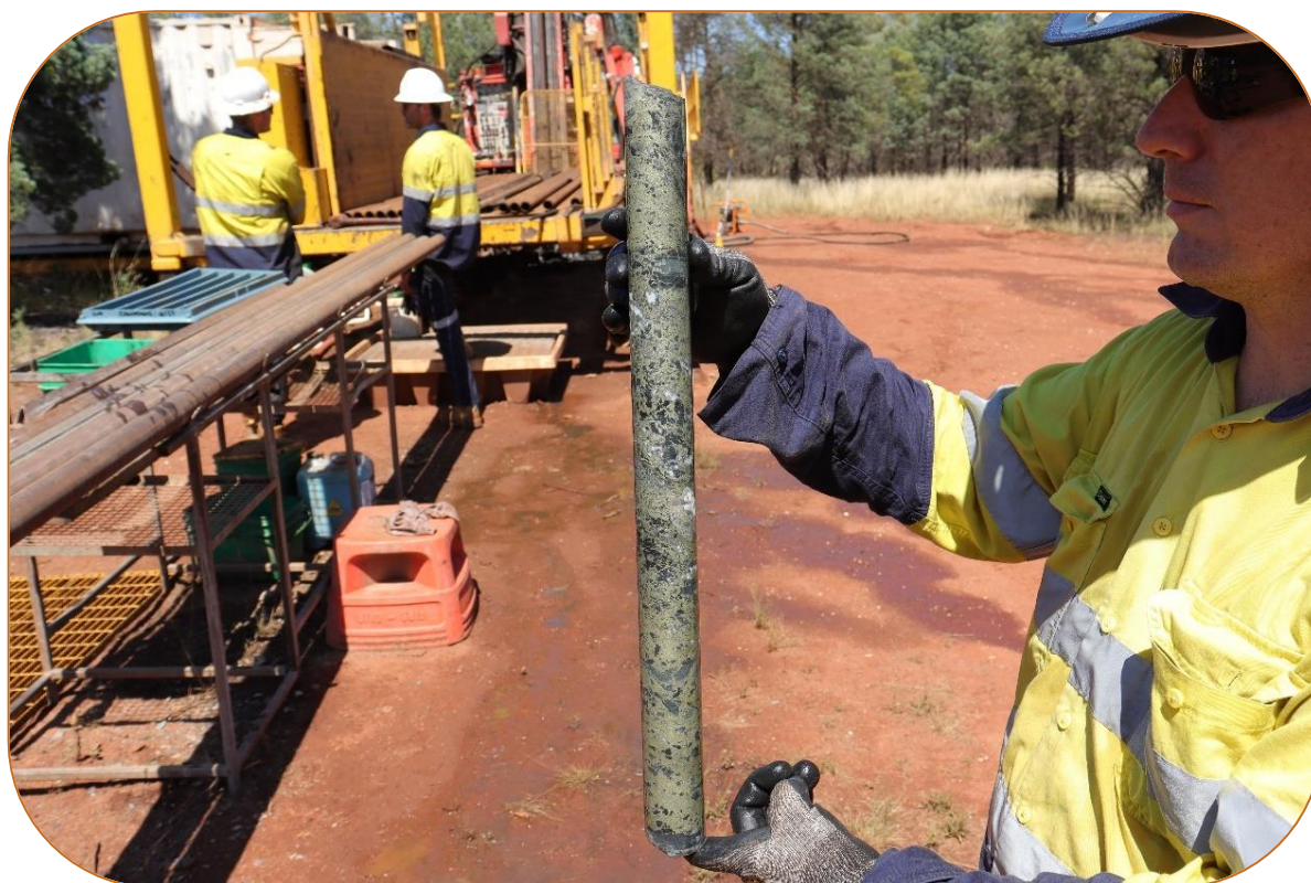
Figure 2 – Massive to semi-massive chalcopyrite intersected from 425.2 metres in CANDD006
