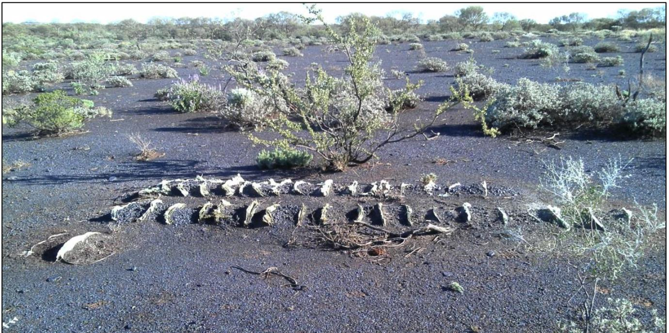
*Figure 10. Drill rig spoil from historic drill hole LRRC03 (EOH 42) with samples laid in rows of 20m*
