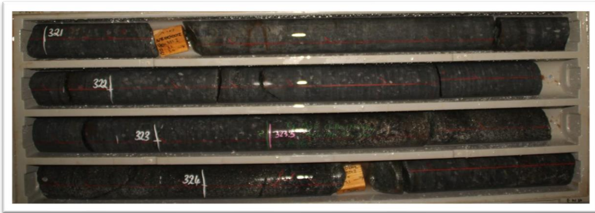
Figure 3 - Diamond Hole NRDD002 (Dry and wet) – Tray #91 - Disseminated sulphide (pentlandite 2%) from 323.3m to 327.4m
