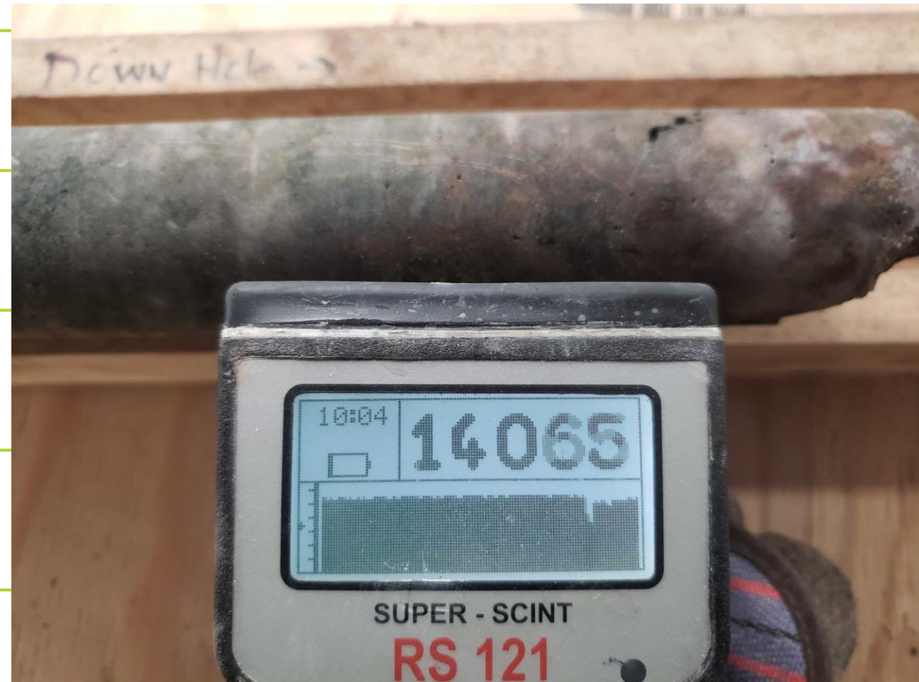
Image: GEM22-019 – RS-121 Hand-held Scintillometer
