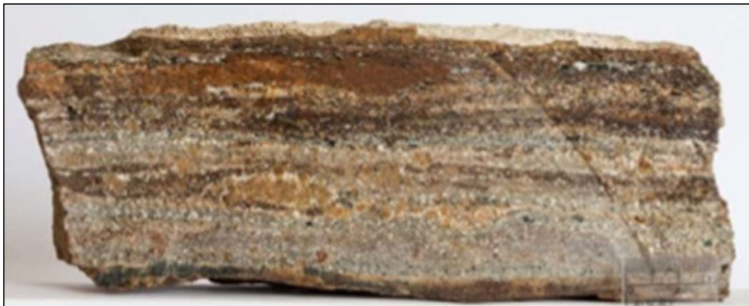
Figure 1: Silver King vein sample showing carbonatite (grey) with rare earth mineralisation (orange-brown)
