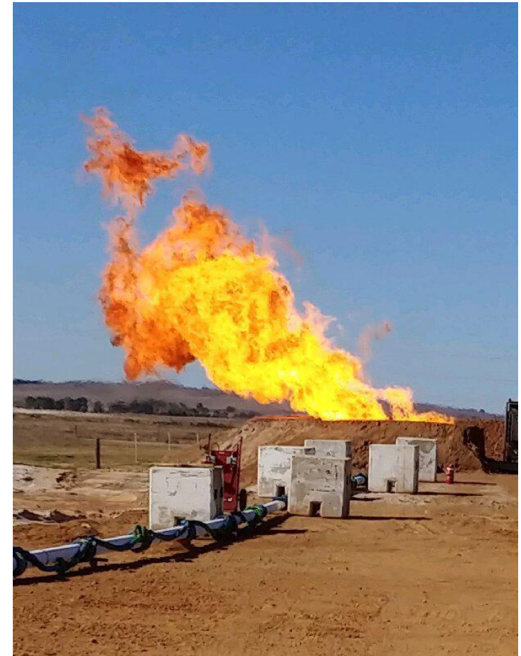
Walyering-5 D Sand flow test
