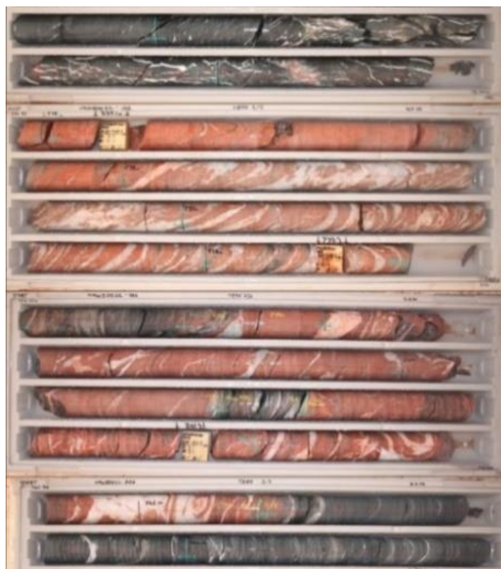
Photo 1: Crusader – Templar Prospect Diamond Drill Hole #6 736m – 740m 4m @ 4.26g/t Au (Within 10.45m @ 1.82g/t Au from 732m) Mineralised, altered and silicified quartz porphyry – “The Right Rocks”
