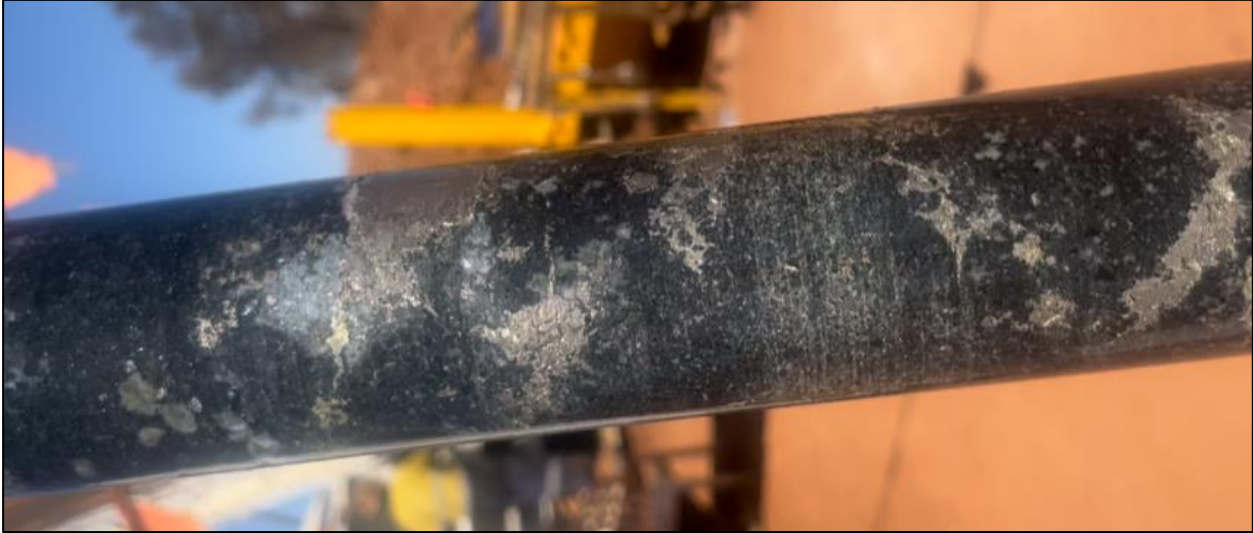
Figure 4: Diamond core with globular nickel-copper sulphides at 802m in CBDD067. Silica plume material is visible in the top row of core with globular nickel-copper sulphides.
