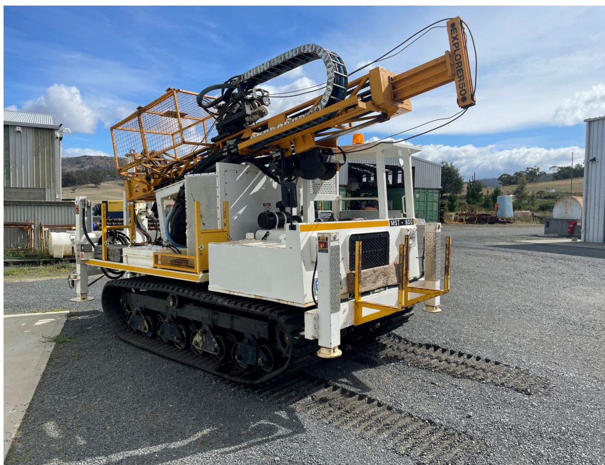
Figure 3: Innovative Hydraulics Explora 50 Air-Core drill
