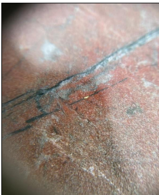
Figure 2: Visible gold associated with chlorite carbonate fracture veins, hosted within a silica, hematite rich mylonite unit – MRDD011 at 151.9 metres
