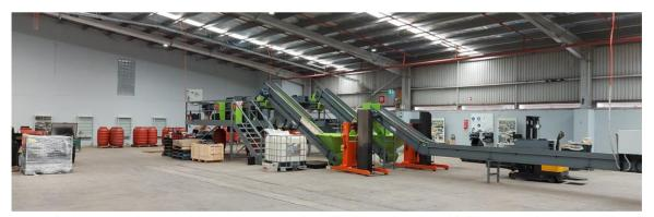
Battery sorting equipment operated by Envirostream in Melbourne, Australia.
