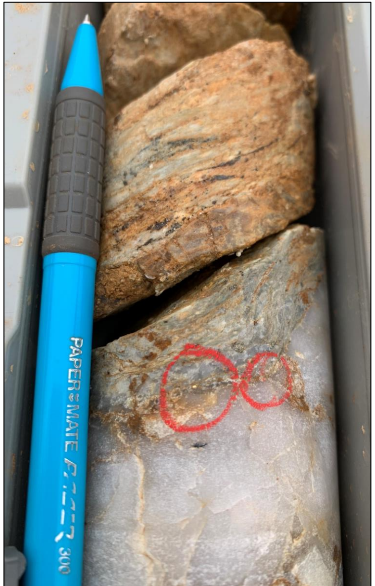
Figure 3 – Visible gold (circled) in drill core from La Mascotte. The gold is located in the quartz-sericite-carbonate alteration selvage adjacent to a thick quartz vein (BLDD220002, 75m) 3 . Cautionary Statement: Visible gold does not provide precise, accurate, or repeatable indications of gold grade. Laboratory assay results are required to determine the widths and grades of any mineralisation reported in preliminary geological logging.
