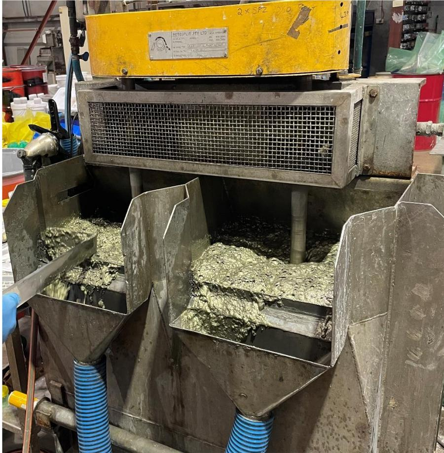
The magnetite test work was announced in “New Environmentally Sustainable Product at Rover” (19 November 2021). In this test, the ore (sized at P<sub>80</sub>106µm) was passed over a Low Intensity Magnetic Separator (LIMS) set at 600 gauss. This magnetic fraction was then reground to 53µm (to meet the specification of the Industrial Mineral). This reground material was then repassed over the LIMS unit and then screened to size fractions to produce the high grade Industrial Mineral.
