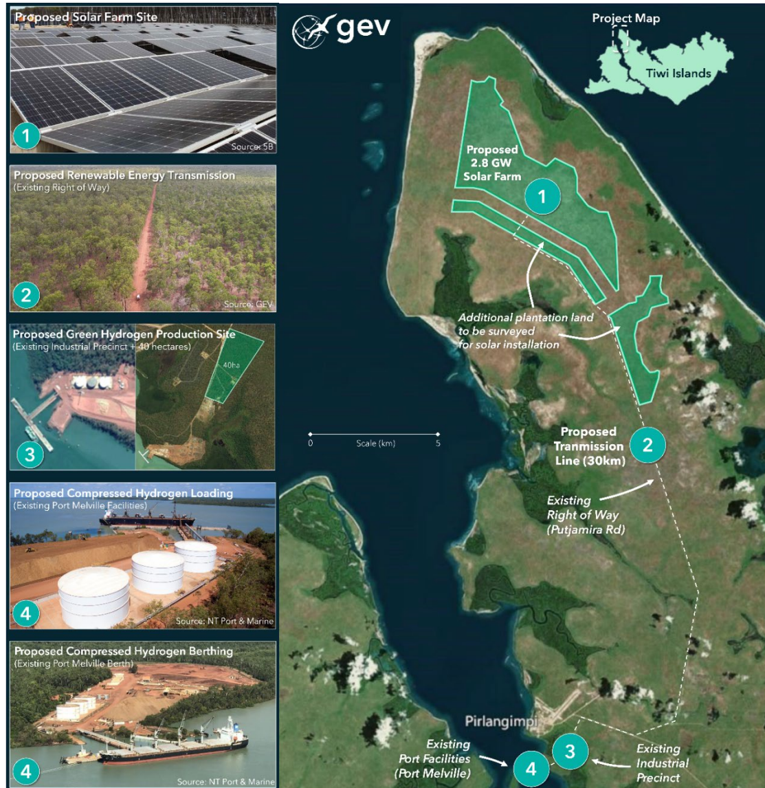
Figure 3: Outline of the Tiwi H2 Project - Including site locations for solar, transmission line, H2 production, compression and existing jetty for loading and export.
