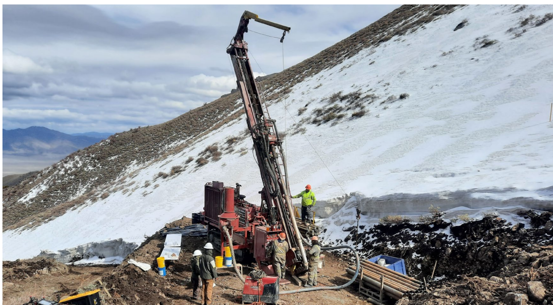
Figure 2 RC percussion drill rig on site drilling the first hole at Star Canyon, Nevada
