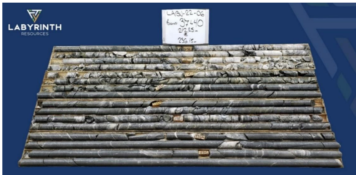
Figure 1 - Core tray containing Boucher intercept from ~213m in LABU-22-06, hosting 7.5m @ 7.01g/t
