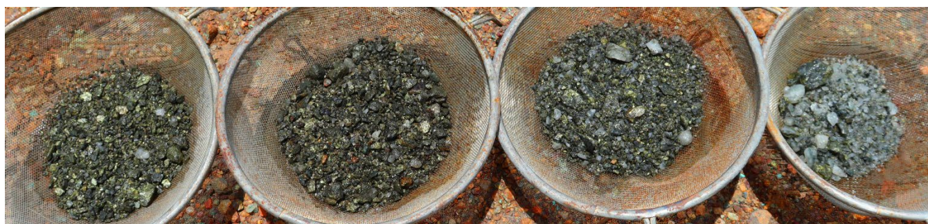
Figure 1. Sieve of sulphidic intervals 27-31m, averaging 6.02% Cu (by portable XRF) in HMLVRC014
