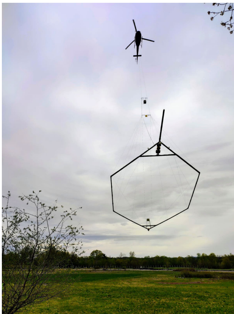
Figure 15: Photograph of the SkyTEM heliborne geophysical survey at Sinjakovo taken on 21 April 2022.
