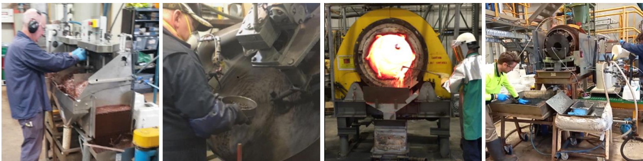
Figure 1 - AVL's process includes reverse flotation, pelletisation, salt-roasting and leaching; demonstrated at full pilot-scale from left-right
