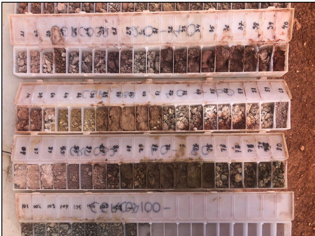
Figure 1: Chip tray for CGRC032 – peak 3.77% nickel value at 74m
