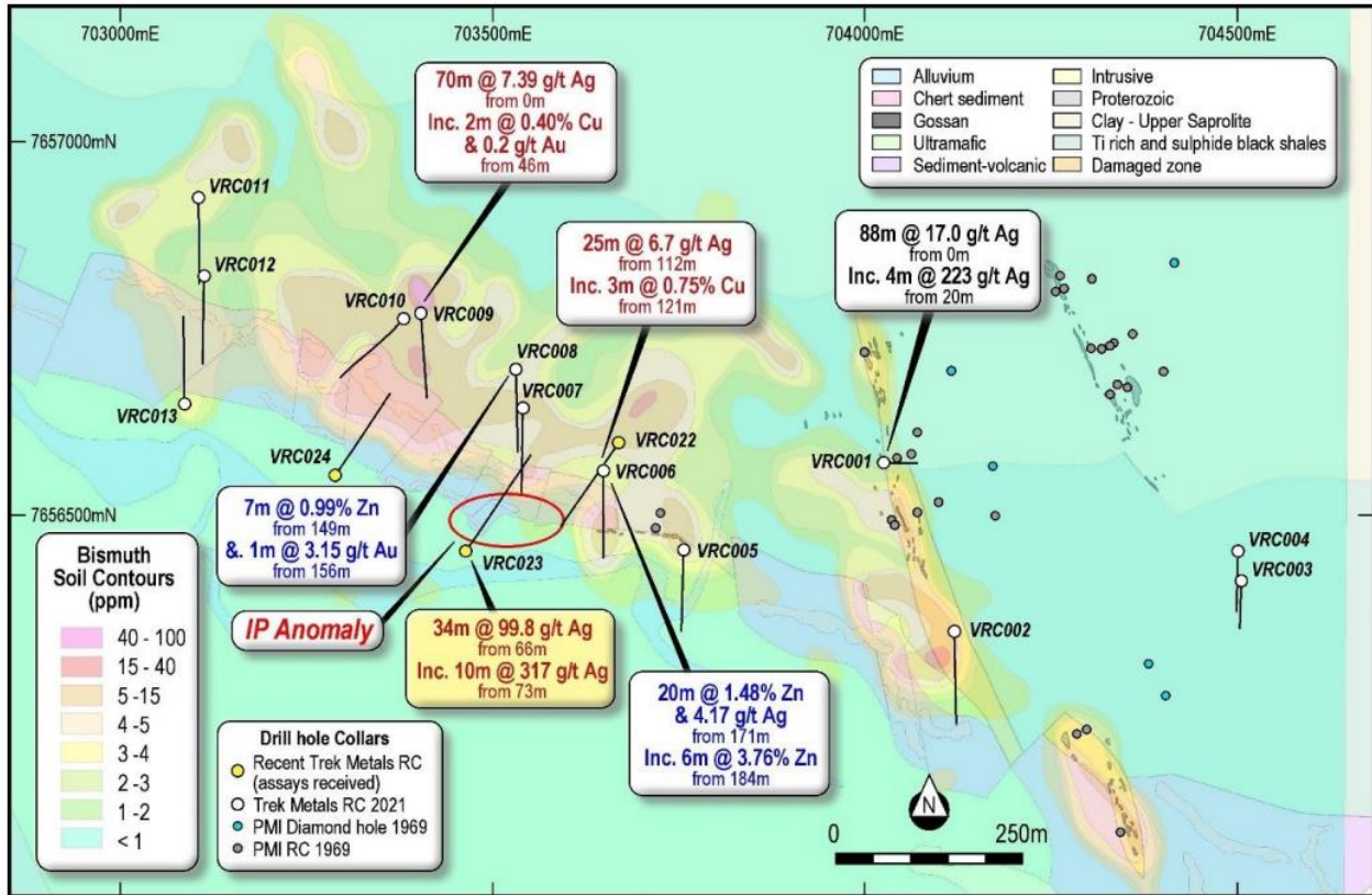
Figure 1: Valley of the Gossans drill collar locations with selected significant intercepts, highlighting the recent high-grade silver intercept in VRC023, which was drilled to test the modelled IP chargeability anomaly.
