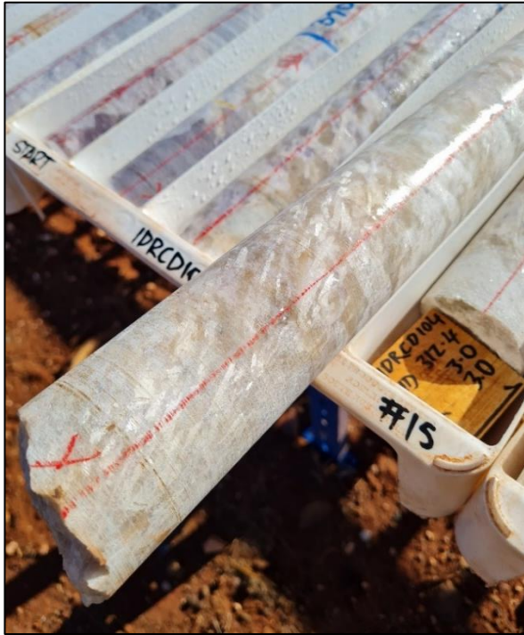
Figure 3; IDRC0104 First diamond core drilled into southern Mt Ida pegmatite 309.4m – 313.4m. The Company has no estimate of potential lithium mineralisation contained within IDRC104 which can only be determined through laboratory analysis.
