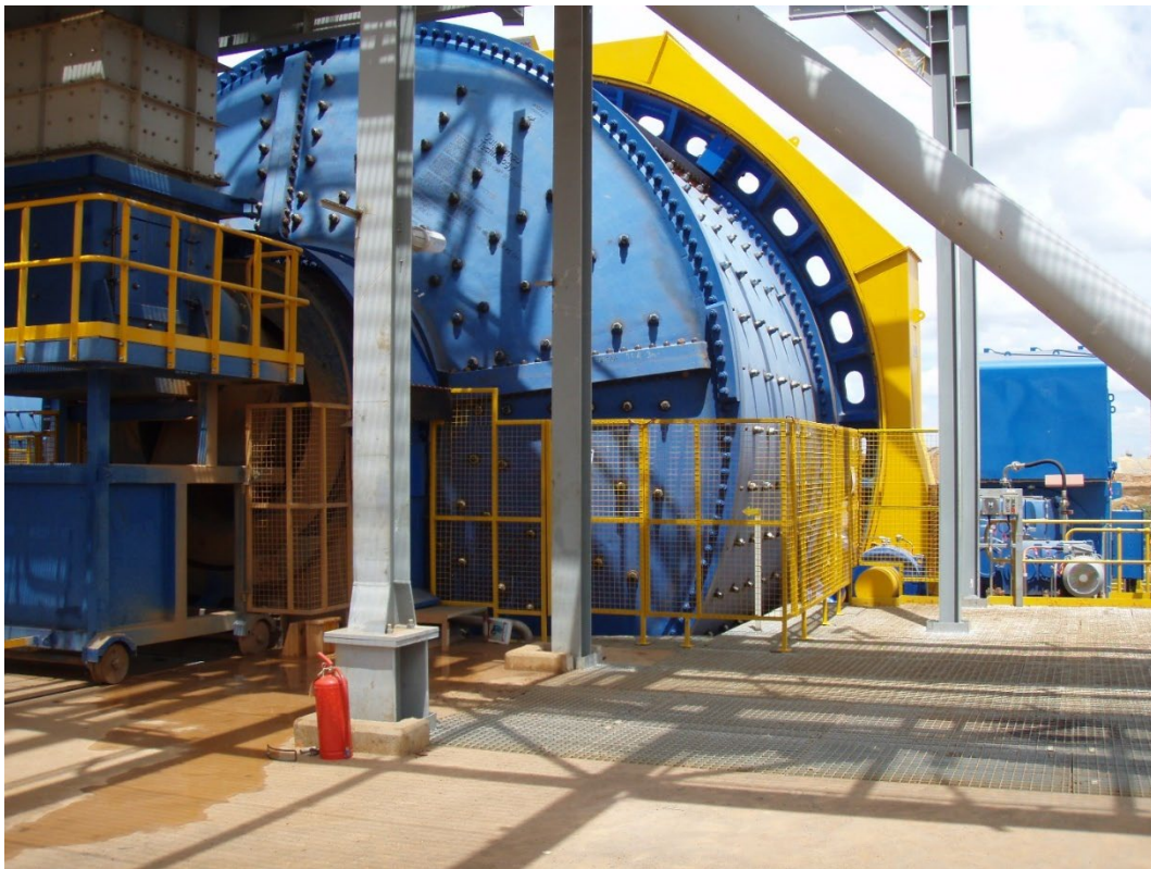
Figure 4: Example of installed Metso-Outotec Premier™ SAG Mill similar to the SAG mill ordered.
