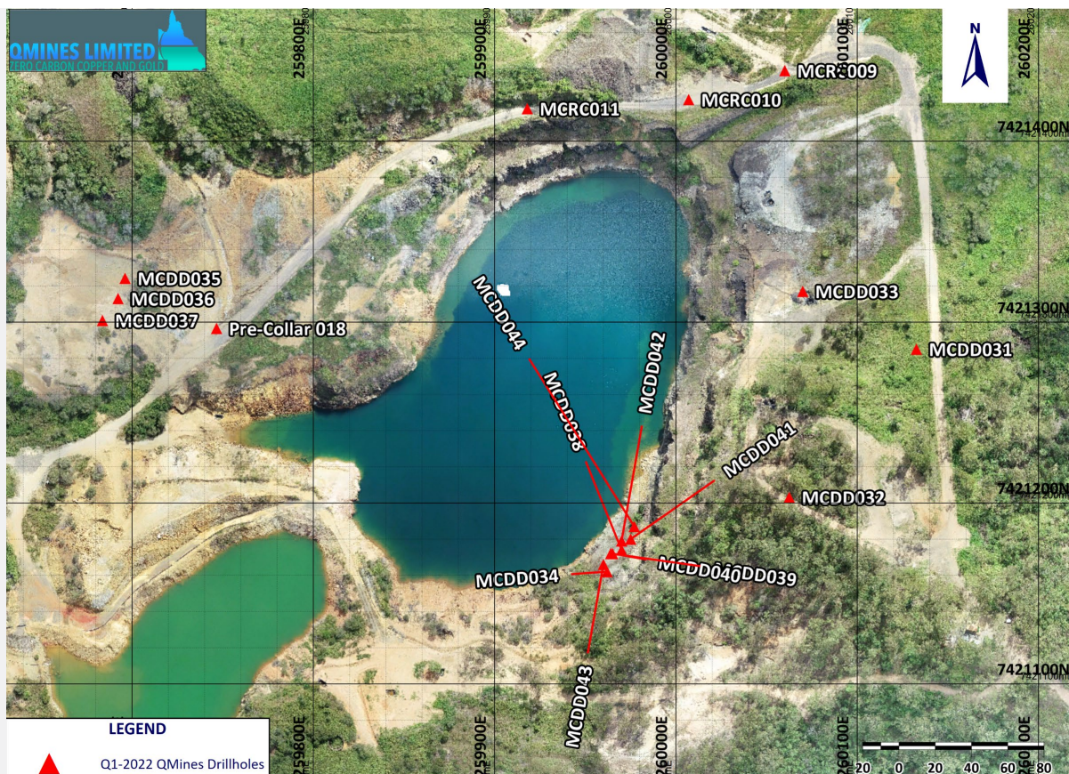
Figure 2: Diamond, RC and RC pre-collar drill hole collar locations, December to March 2022, Mt Chalmers project.
