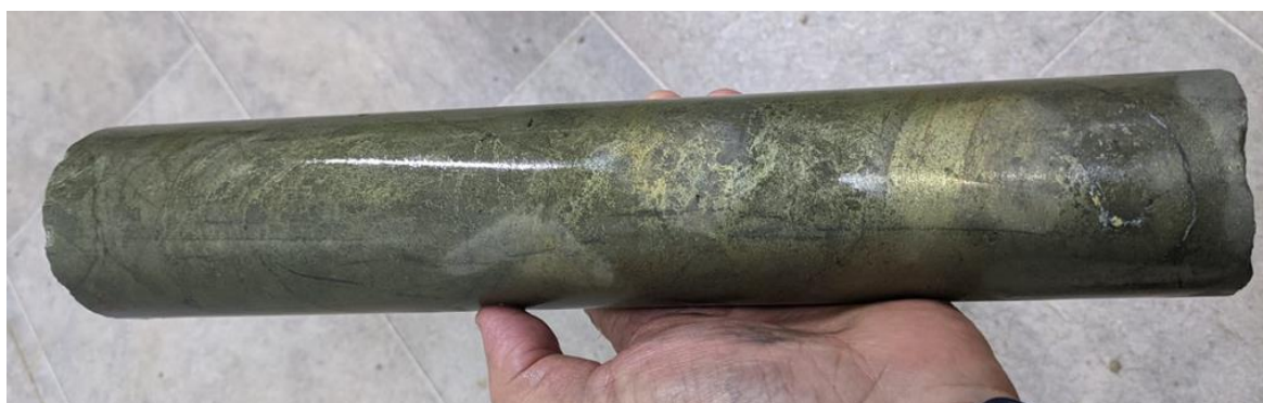
Summary Image 2 –21DMDD03 Massive chalcopyrite, sphalerite, pyrite intersection from 145.95m.
