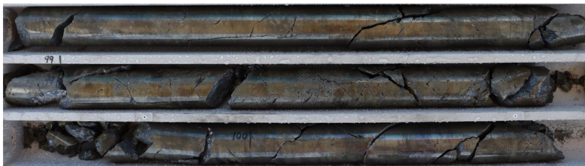
Summary Image 1: 22DMDD09 98.95-101.5m Massive pyrite chalcocite with minor relict chalcopyrite, bornite and sphalerite.
