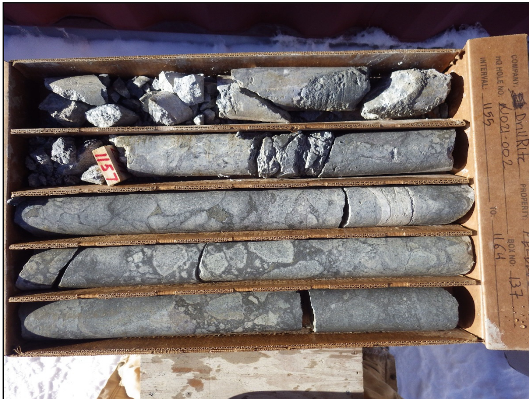
Figure 2. Brecciated unit in hole 21ND_002 showing altered andesite clasts within a pyrite-rich matrix (from 1155 to 1164ft (352 to 354.8m))
