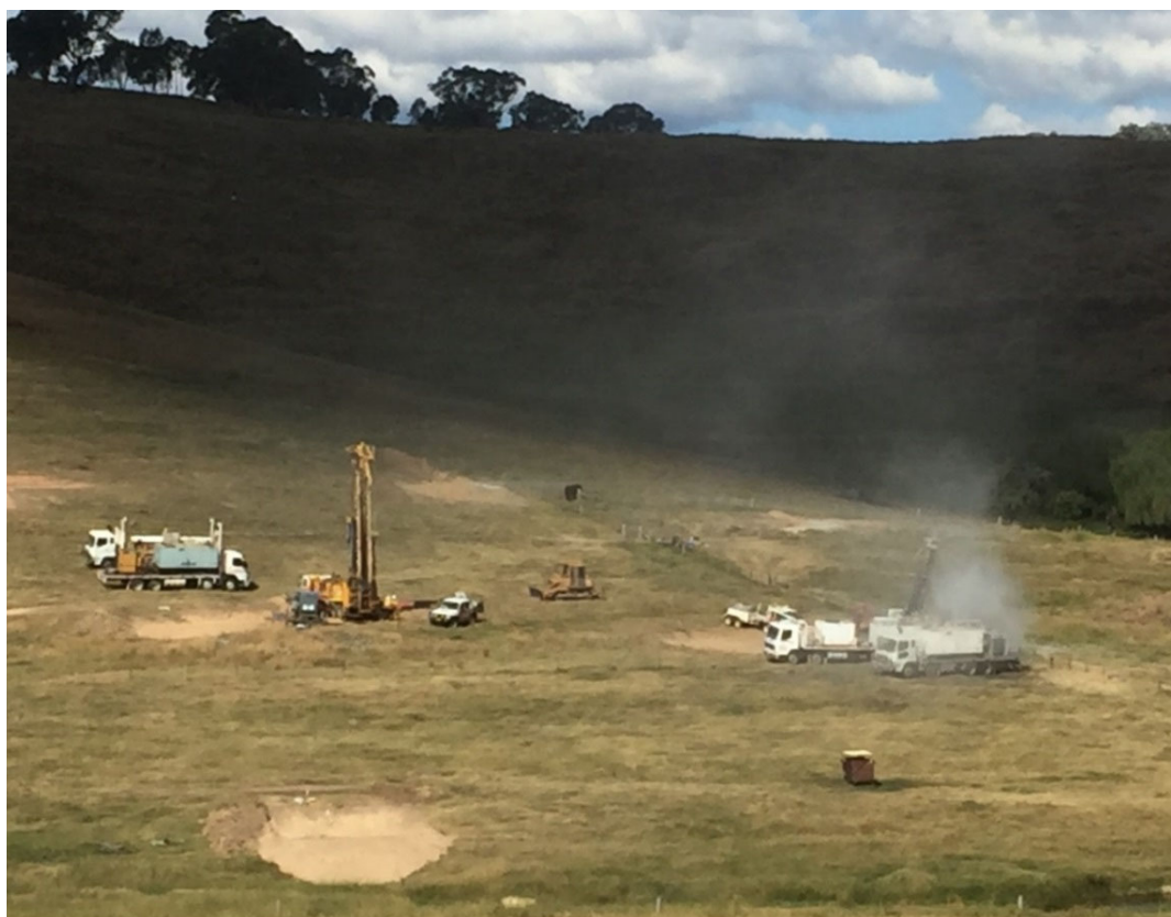
Figure 3: Track mounted Rig (right) drilling hole CAL004 while the Truck mounted Rig setting up to drill. Several drill pads also prepared for drilling.
