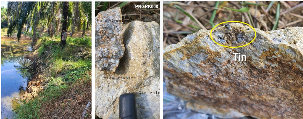
Figure 4: Phang Nga sample PNGRK008 from a water course cutting showing tin mineralisation
