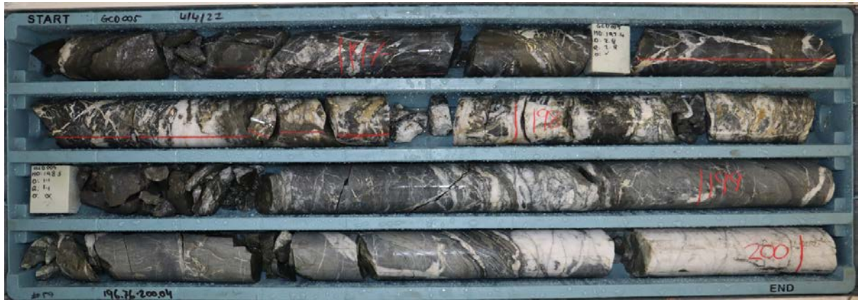
Figure 6: Golden Camel diamond drill core from hole GCD005 showing sulphide mineralisation and substantial brecciation.
