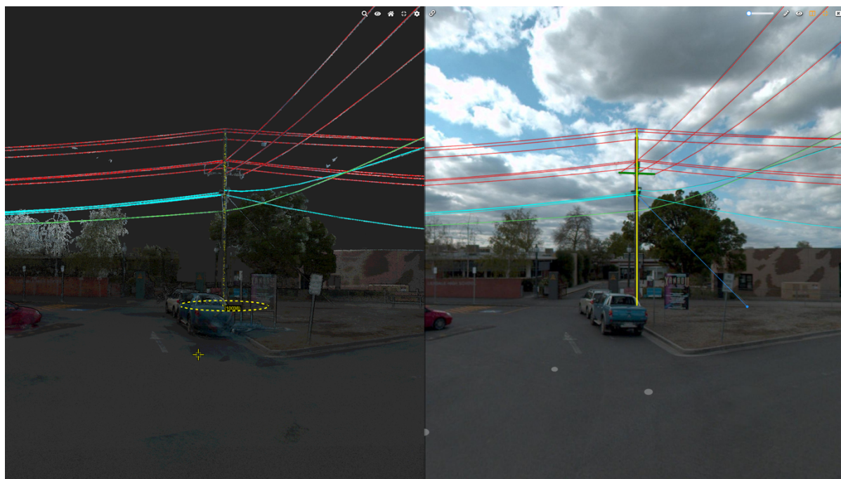
Image above shows synchronised view of a Pointerra poles and wires digital twin model overlaid on the point cloud (left) and the panoramic imagery (right)
