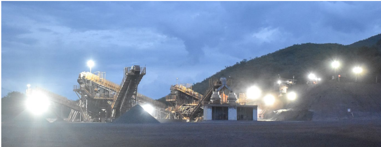
Figure 1 – A Tertiary Crushing Circuit was added in the December Quarter
