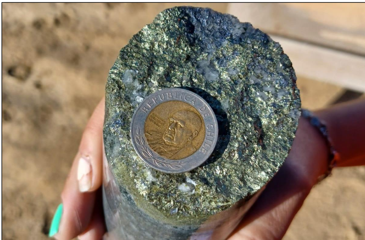
Figure 3: Core from CMLCD001 with Cu and Mo sulphides, refer Appendix D, (150-151m downhole). The visible mineralisation is based solely on a visual inspection and has not been assayed.
