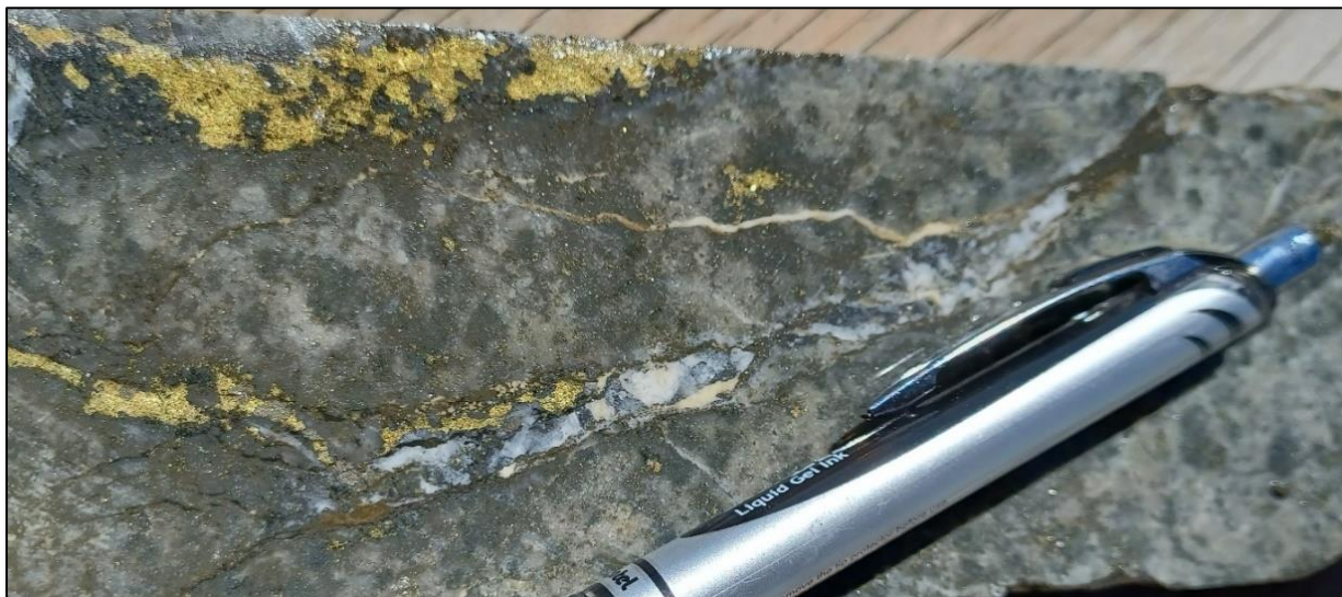
Figure 2: Lana Corina copper sulphide mineralisation (Drillhole LCD – 13: 2.05%Cu, 20ppm Mo From 330 – 331m) (ASX announcement 21 March 2022). The visible mineralisation is based solely on a visual inspection and has not been assayed.
