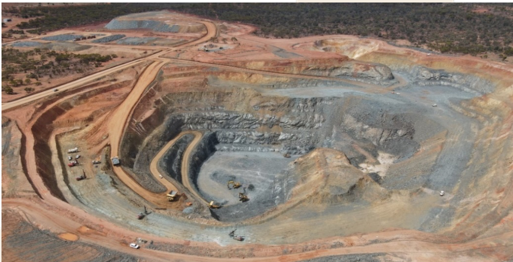
Figure 2 – Missouri mining operations showing Stage 1 (centre) surrounded by the larger Stage 2 cutback
