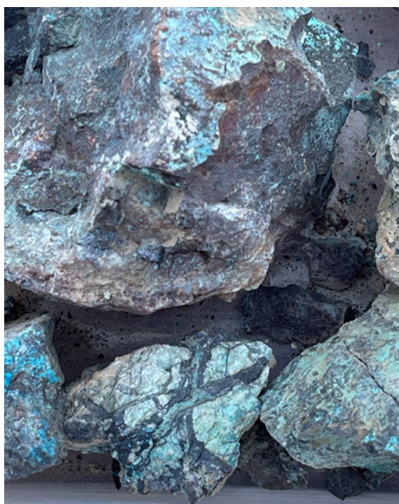
Figure 3. Sample NSM-21-032: 16.8% Cu and 8.48g/t Au (772413E, 3781087N)
