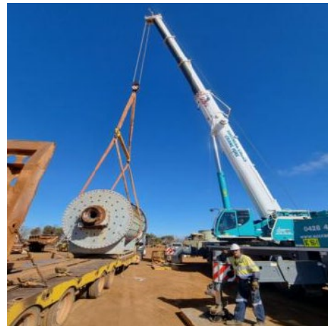
Spare ball-mill at FNO being transported to Perth for refurbishment and re-use at Cosmos operations.
