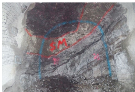
641 south ore drive (4.0mW x 4.5mH) with a face grade 2.5%
