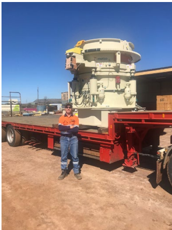
Secondary Crusher delivery onsite
